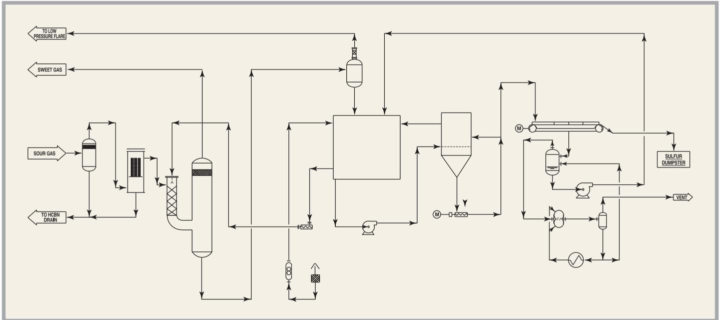
of 60,000 to 100,000 normal cu m/hr, with a sulfur load of about 50 kg/day (due to low H<sub>2</sub>S concentration in the gas). Current H<sub>2</sub>S removal efficiency is 90%, producing gas suitable for pipeline quality.
