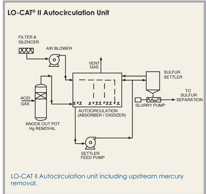
The LO-CAT<sup>®</sup> II process offers a low-cost, high-efficiency, flexible method for removing H<sub>2</sub>S from geothermal non-condensable gases achieving 99.9+% H<sub>2</sub>S removal efficiency.
