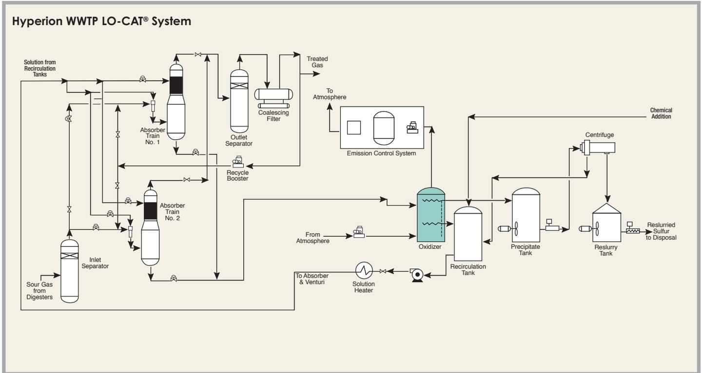
LO-CAT worked with the City to design the plant modifications required by the LO-CAT<sup>®</sup> Process. The existing packed columns were converted to Mobile Bed Absorbers (MBA). The remaining process was essentially unchanged from the original Stretford design. The Stretford practice of floating sulfur for separation was even retained. Outwardly, the unit looks the same; the only difference is the catalyst.
